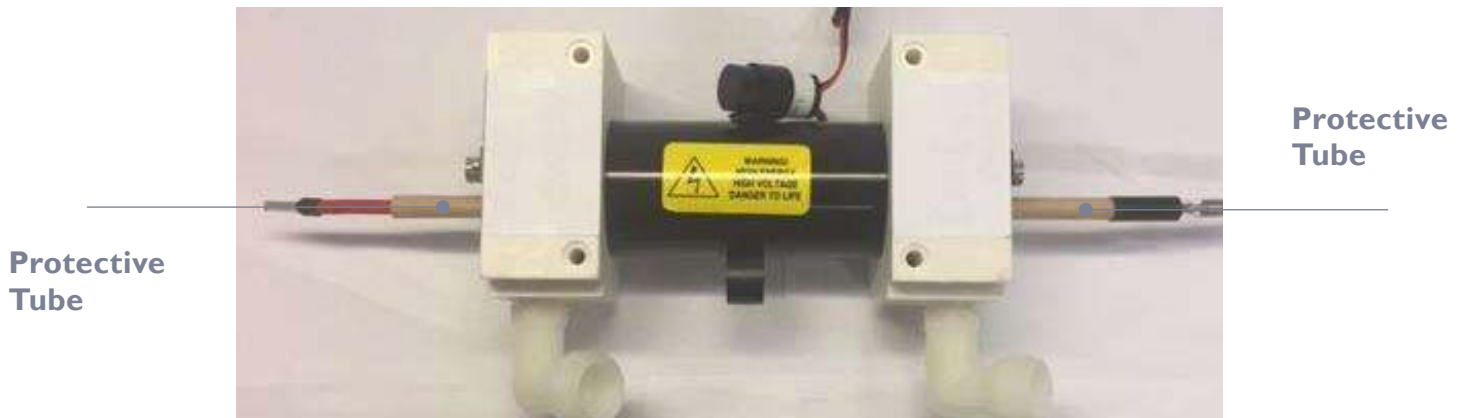
Figure 10 (Flashlamp Installation [with Protective Tubing & Plastic Ends Equally Extended])
