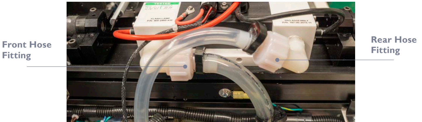
Figure 20 (Connect & Tighten the Hose Fittings [x2 total])
