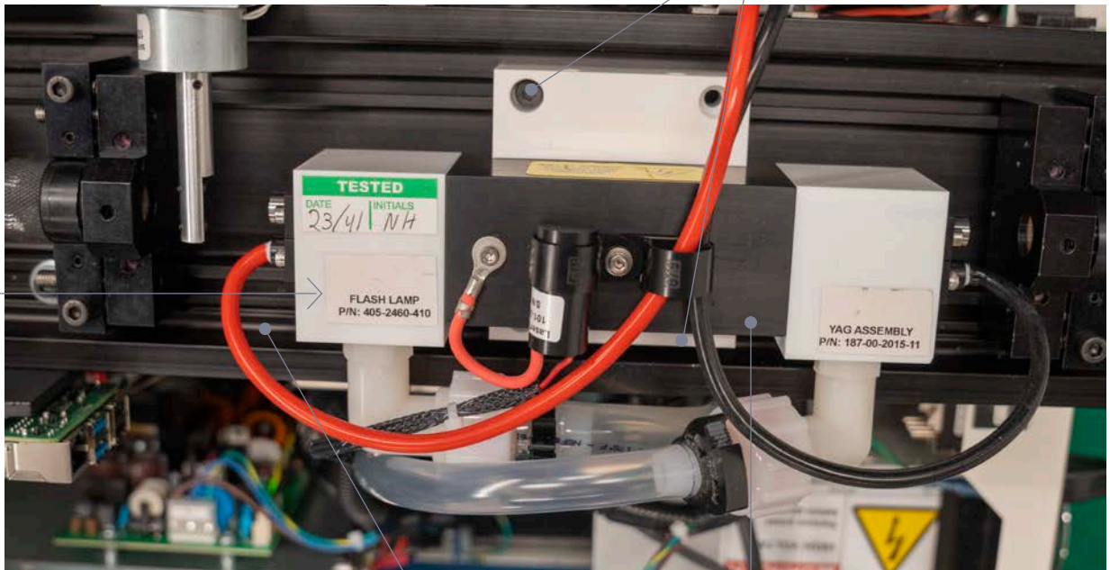
Figure 16 (Pump Chamber [Positioning the Assembly Against the End Stop & Optical Rail Reference Edge])
