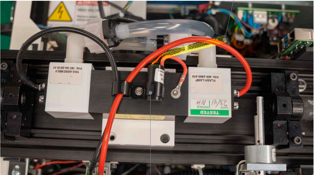
Figure 2 (Disconnect Flash- lamp Wires; Left Side View of Laser Rail)
