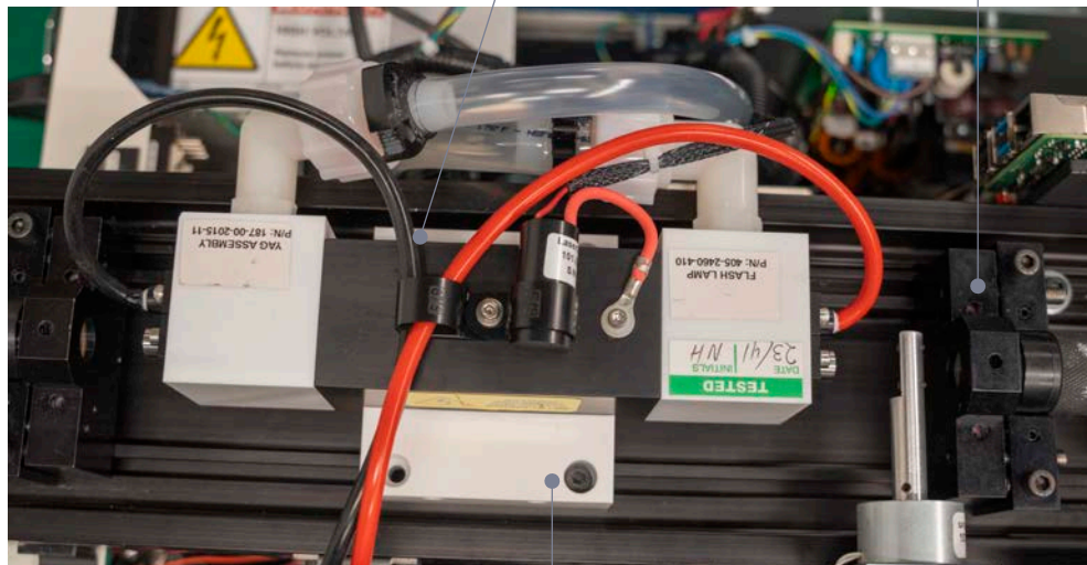
Figure 15 Pump Chamber [Installation] & Fastening the Screws to the Optical Rail)
