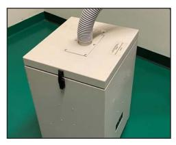
19. Connect the exhaust hose and then connect to the exhaust unit and rear of the lasing chamber, as shown. Be sure to properly position the interior chamber adjustable exhaust tube to the required lasing area to ensure maximum suction.
