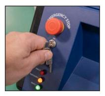
17. Locate and open the box labeled "accessory kit" and retrieve the following items: keys, remote interlock, power cord, USB hub, and USB cables.
