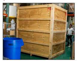
5. Cut and remove the straps of the boxes alongside the laser system and carefully remove the boxes.
