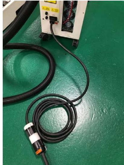
Figure 3 (8801 Series; Laser Engine Power Cable)
