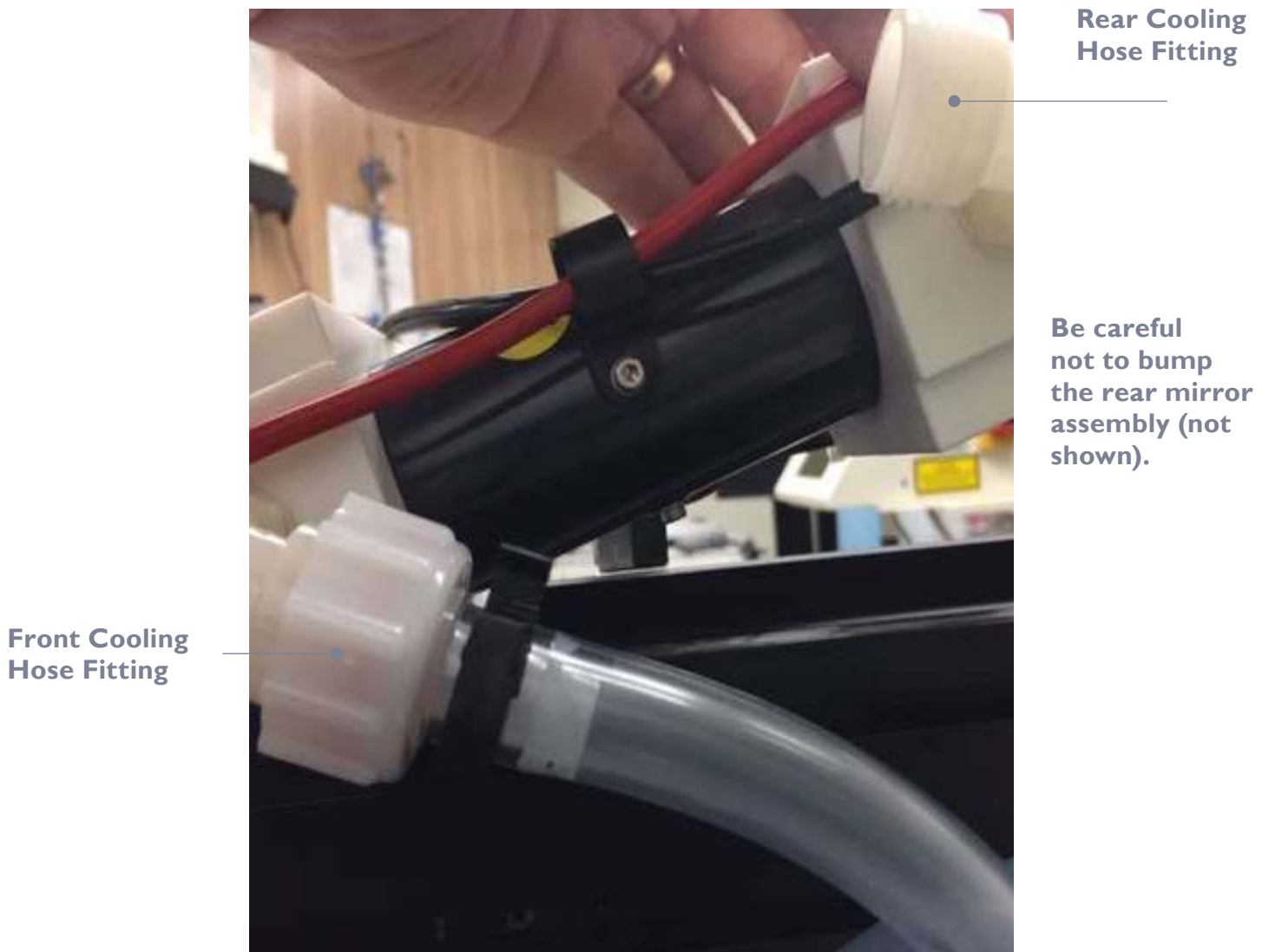
Figure 5 (Pump Chamber [Tipping & Draining])
