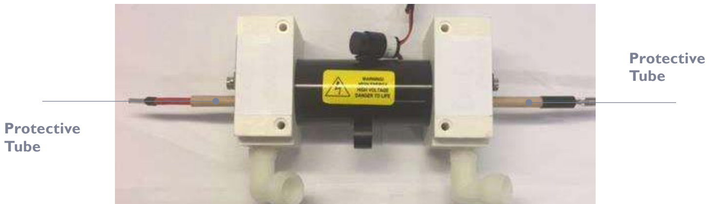
Figure 9 (Flashlamp Installation [with Protective Tubing & Plastic Ends Equally Extended])
