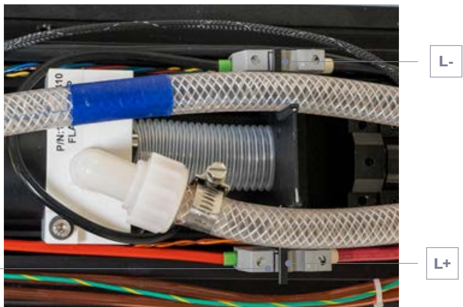
Figure 19 (Flashlamp Wires; [Optical Rail; top view, back side])
