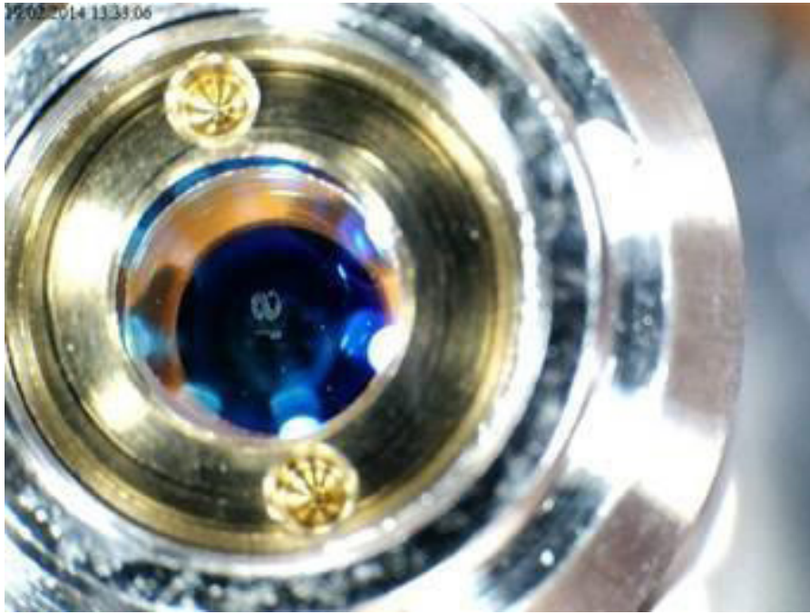
Figure 1 (ILLK optic; Etch damage from back- reflected light)
