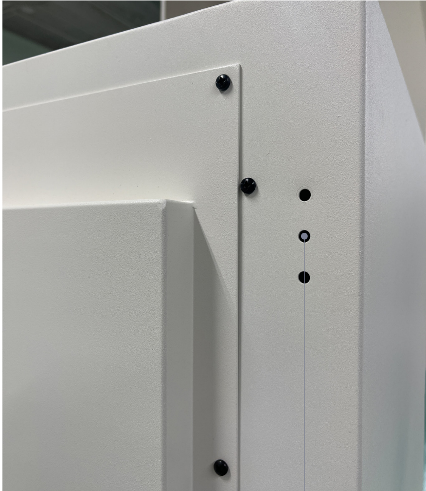
Figure 2 (Removing the counterweight securing bolts)
