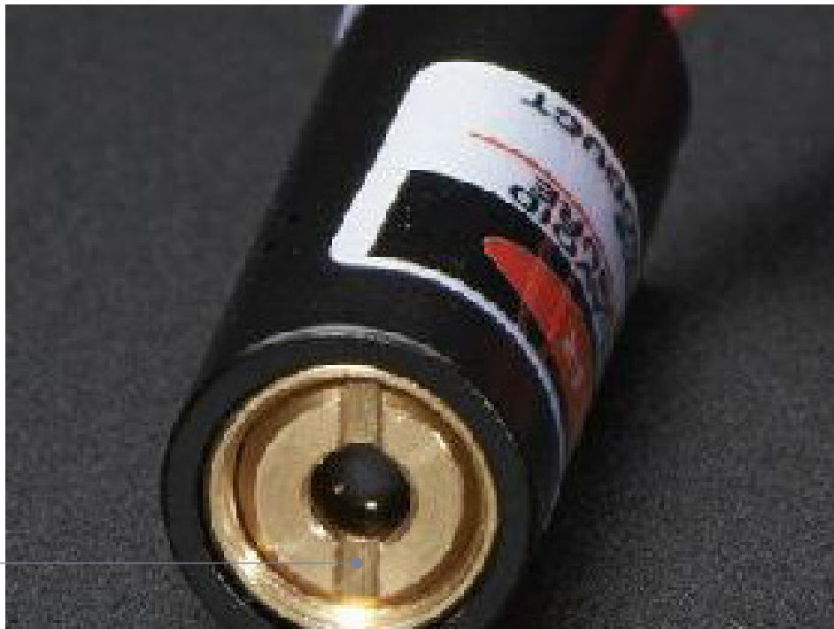
Figure 4 (Focus diode; adjustment slot)
