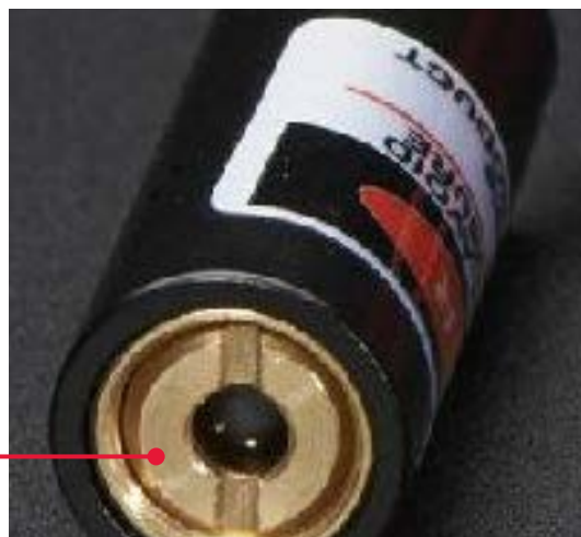
Figure 5 (Focus diode; adjustment slot)
