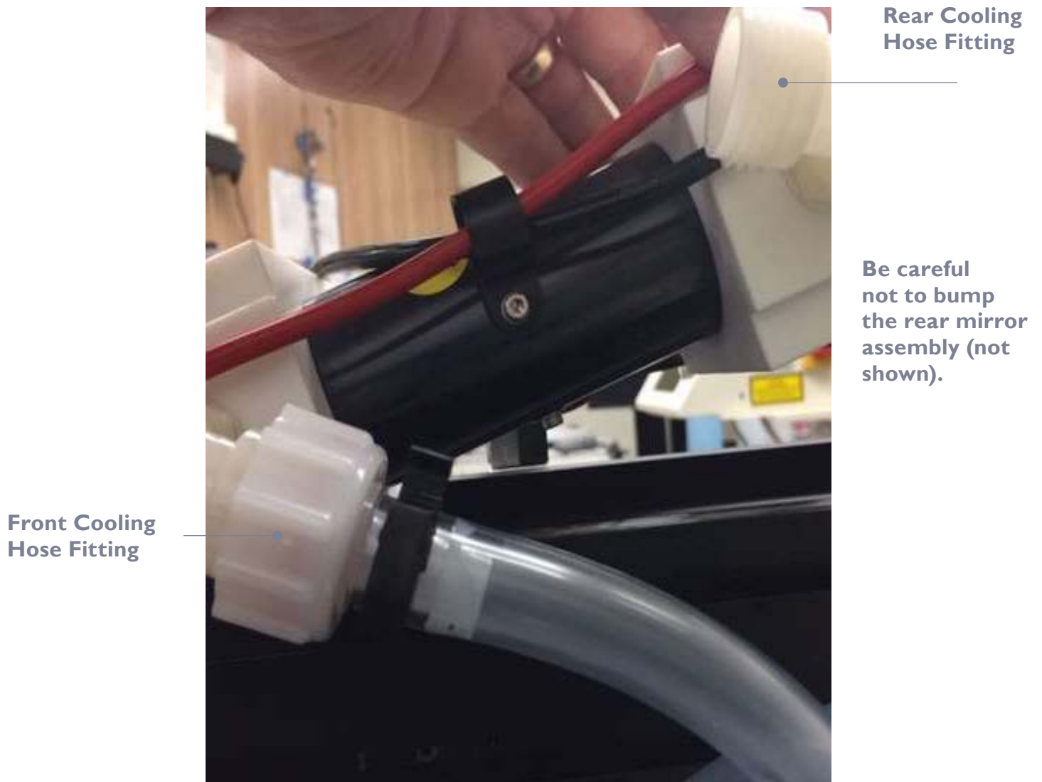
Figure 5 (Pump Chamber [Tipping & Draining])
