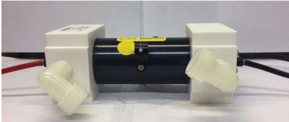
Figure 6 (Pump Chamber [with Flashlamp Wires Removed from the Cable Clamp & Straightened])
