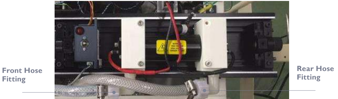
Figure 21 (Connect & Tighten the Hose Fittings [x2 total])
