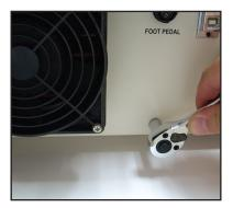
**6.** With the slotted side of the bracket facing toward the laser welder, thread the bolt into the hole, and use the socket wrench to secure the brackets to the rear of the laser.
