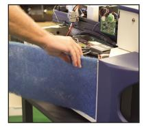
12. Locate the distilled water tank (rear of the iWeld) and open the container by unscrewing the top cover. Pull the top cover and attached filter upward carefully; remove and set aside. (Warning: Make sure that your bare skin or fingers do not touch the water filter.)
