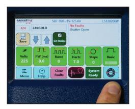
29. Depress the **Arrow buttons** on the touch screen and select memory cell #24/24 CROSS-HAIR ALIGN by using the **Up** or **Down Arrow buttons**.
