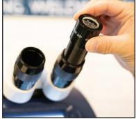
**26.** If the operator does not wear eyeglasses, you may insert the rubber eye cups on the ends of each ocular.
