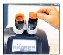
25. Remove the oculars from the box and place one in each eye tube. (Note: One ocular is marked with a "+;" place this ocular into the tube of the operator's dominant eye—usually the right eye.)
