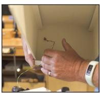
10. Remove the left-side cover from the machine by unscrewing the six (6) cross-head screws positioned along the sides of the panel. (Note: A manual screwdriver works best.) Move the cover away from the machine and disconnect the grounding cable (located on the inside top of the cover); set the cover aside.
