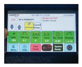
**30.** Depress the **Set Recipe** button (yellow button; located in the center of the touch screen). The parameter buttons will all turn green.
