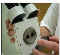
24. Place the flange into the mounting ring at the top front of the laser. Retrieve the 2mm Allen wrench (provided). Holding the scope facing forward, tighten the two (2) mounting screws (located on the mounting ring at 5 and 7 o'clock). When the scope is securely mounted, remove the rubber tube protectors.
