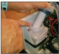
13. Using a clean funnel, siphon hose or by carefully pouring directly, fill the distilled water tank with the distilled water (provided) to the black site line (max – filter out) marked on the side of the tank. (Warning: Make sure the water does not come into contact with the electrical components.)
