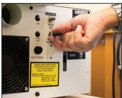
21. Retrieve the foot switch from the accessory kit. Plug the cable into the outlet marked "Foot Pedal" (located on the rear of the laser) and turn the threaded fastener to tighten. Place the pedal on the floor.
