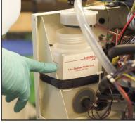
**14.** Replace the top cover and filter for the distilled water tank. Next, verify that both the **Mains Power** Switch and Key Switch are "OFF."
