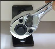
**7.** Securely fasten the brackets to the tabletop using the appropriate anchor bolts or screws.
