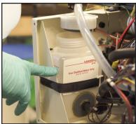
18. Turn the Mains Power Switch "ON" and allow the laser to run for about 5 minutes (or until there are no more bubbles cycling through the water lines). Check the water level in the distilled water tank and fill with additional water, as needed.
