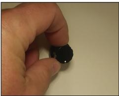
If the laser is equipped with a ring lamp, the lamp has been previously installed, and you can proceed with powering up the machine by turning "ON" the key switch; this will power up the ring lamp. (Note: If the ring lamp does not power up, turn the black knob [inside the chamber] clockwise until it turns on.)
