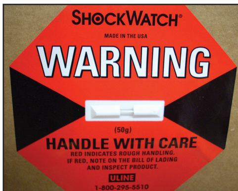
Tube is not red: (no shock warning)
