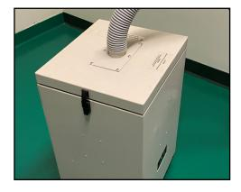
**30.** Connect the exhaust hose and connect to the exhaust unit and the rear of the lasing chamber, as shown.
