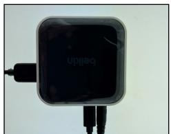
**24.** Plug the mini USB cable (supplied with the hub) into the USB hub. Plug the other end of the cable into a USB port on the computer.
