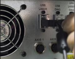
**20.** Aqcuire and feed all of the wires and the pendant out of the back of the enclosure as seen below. This is in order to connect the system to the necessary outlets and to easily access the pendant.
