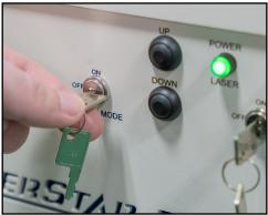
27. Remove the foam block by pressing the UP button; the z-axis will begin to shift upward. Continue to press and hold the UP button until the focus head is raised 2" to 3". Now, carefully remove the foam block. (Caution: When removing the foam block, do not press the Down button; shifting down will damage the focus head and focus lens component.)
