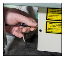
**17.** Retrieve the remote interlock component and insert it into the rear input labeled "remote interlock" (note the notched alignment).
