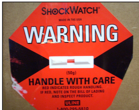
Tube is red: (shock warning)
