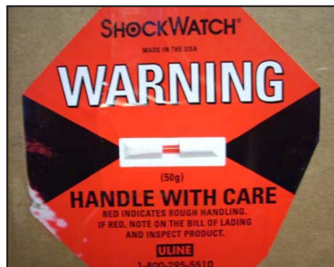
Tube is red: (shock warning)
