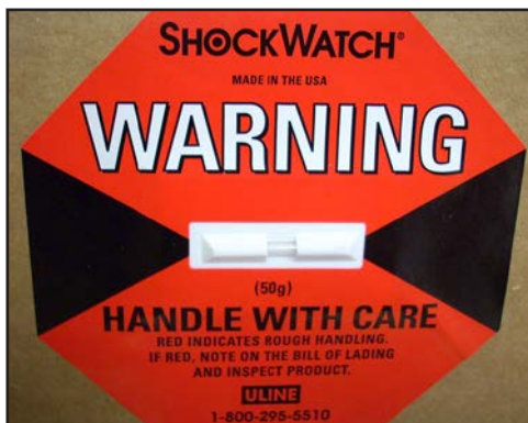
Tube is not red: (no shock warning)
