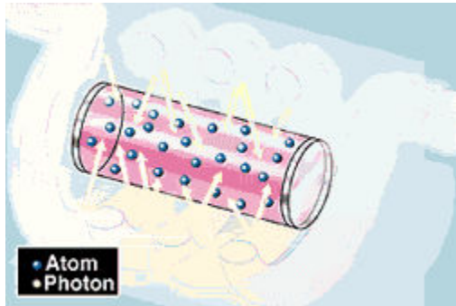
Fig. 4 High-voltage electricity causes the Flash Lamp to emit an intense burst of light, exciting some of the atoms in the crystal to a higher energy levels.
