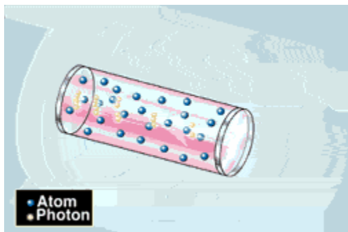
Fig. 6 Mirrors at each end reflect the photons back and forth, continuing this process of stimulated emission and amplification.
