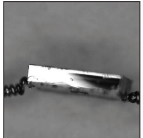
.003" Wire Welded to .003" Platinum
